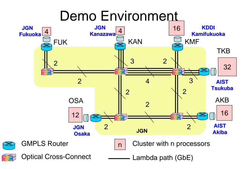
Clusters distributed over six locations in Japan are connected over GMPLS network test-bed deployed by JGN II
